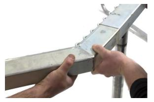
Step 1.3.1 Ensure the steel join is fully inserted, as shown.
