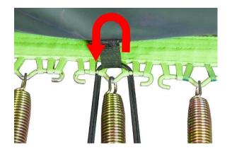
Thread the bungee up through the mat, pad's attachment loop and down through the mat (on the other side of the spring). **Note:** Ensure the bungee is routed in between the mat loops like shown in the picture.
